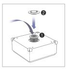
5 Turn over the 'Dust Collector' and replace the HEPA filter at the bottom as well.
