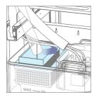
When using this function, position the 'Water Drainage Hose' from the 'Filter box' to the 'Cleaning Water Box'.
