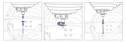
4 Clean the inside of the spindle using the 'Cleaning Cotton (Spindle)' from the service kit.
